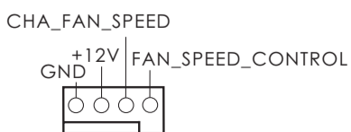
7 : 4-Pin Chassis FAN Connector (+12V)
