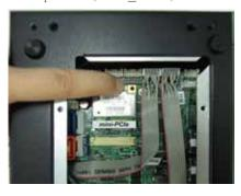
2. Tighten the screw that holds the card in place.
