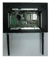
3. Set the WiFi 2.4/5 GHz Antenna at 90-degree angle.
