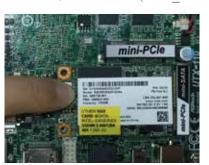
2. Tighten the screw that holds the module in place.
