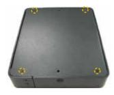
2. Remove the two screws on each side.
