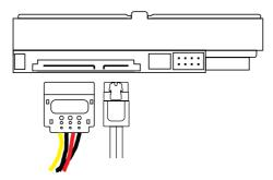
STEP 3: Connect the other end of the SATA data cable to the mother-board's SATA2 connectors.
