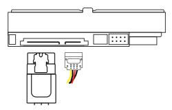
STEP 3: Connect the other end of the SATA data cable to the mother-board's SATA connectors.
