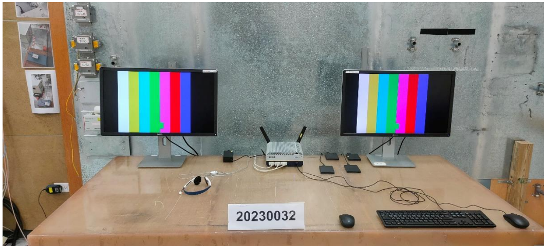
Conducted Emission Test Set up-Front View of Power Ports
