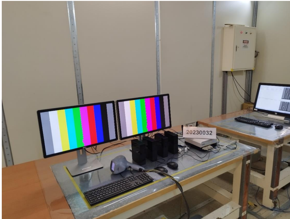
ESD Test Set up-Front View
