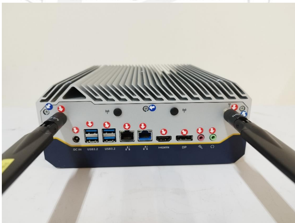
Air and Contact Discharge Test Point-Rear View
