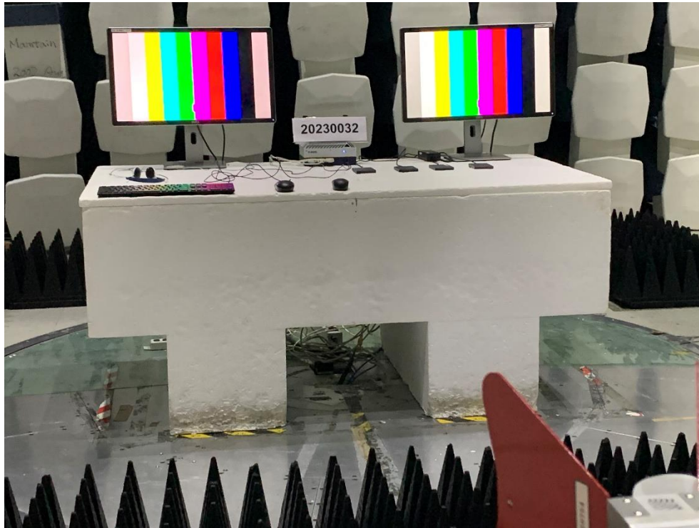
Radiated Emission Test Set up(Above 1GHz)-Front View
