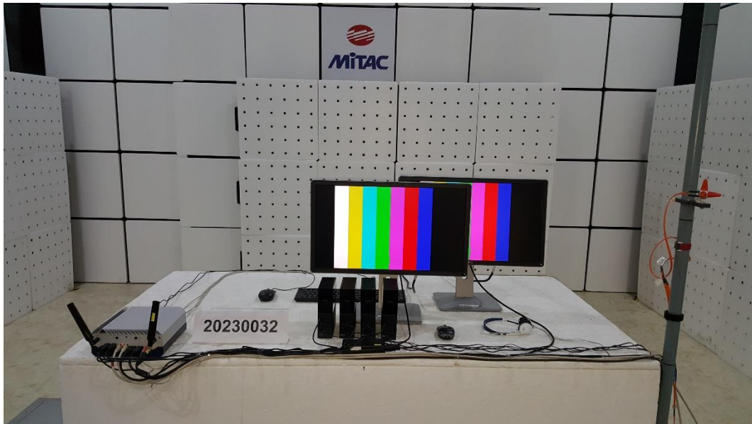
Radiated Susceptibility Test Set up-Front View
