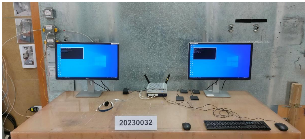
Conducted Emission Test Set up-Asymmetric mode(1Gbps)
