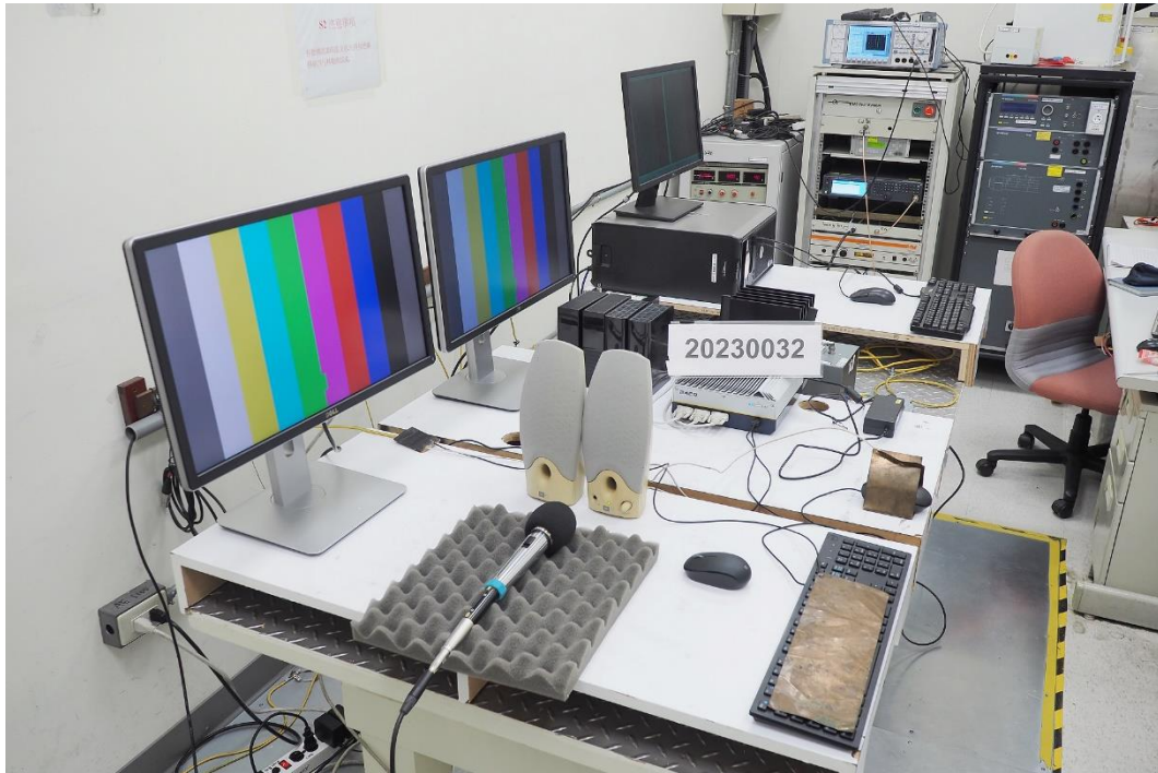
Conducted Immunity Test Set up-Front of Power Port
