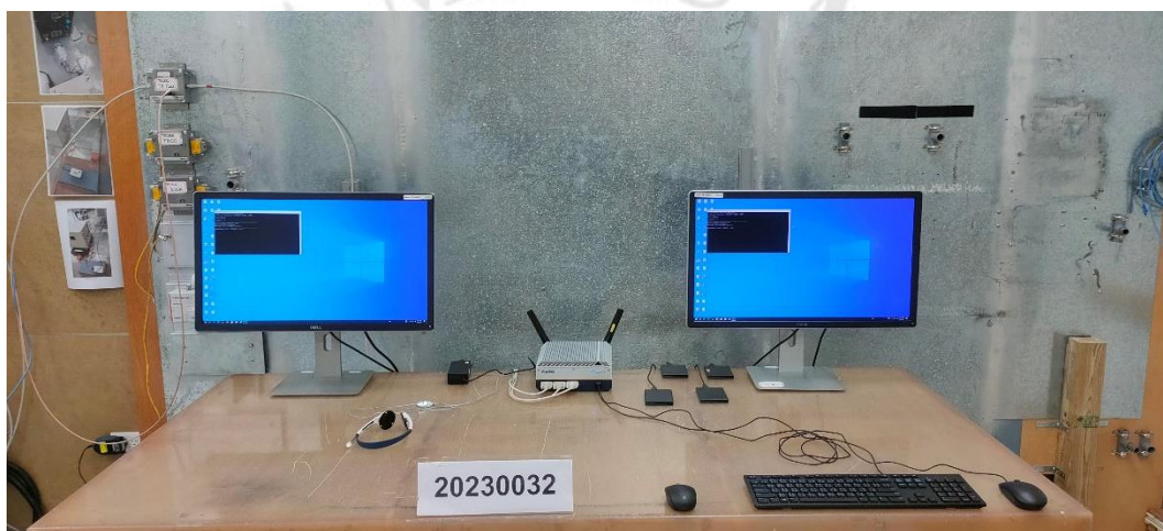
Conducted Emission Test Set up-Asymmetric mode(2.5Gbps)
