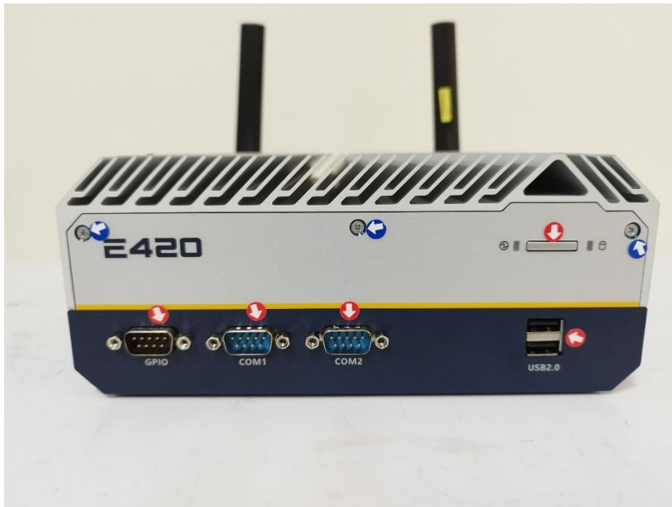
Air and Contact Discharge Test Point-Front View
