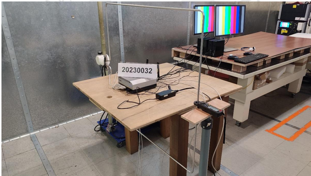
Power Frequency Magnetic Field Test-Vertical View
