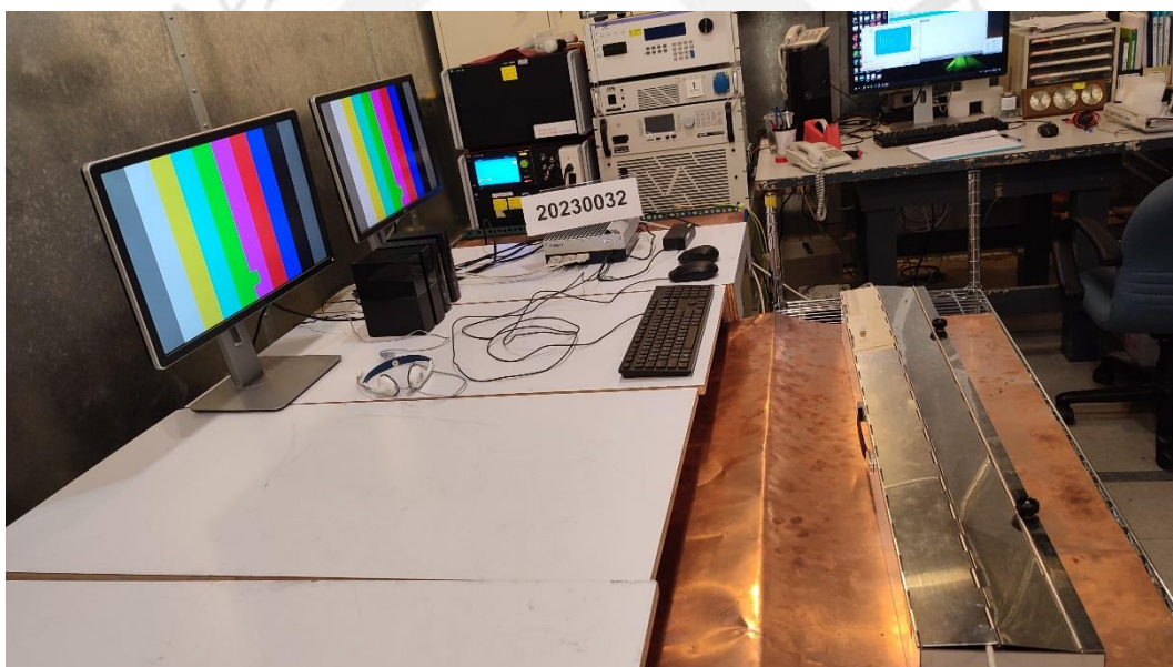
Electrical Fast Transient/Burst Set up-Signal Port
