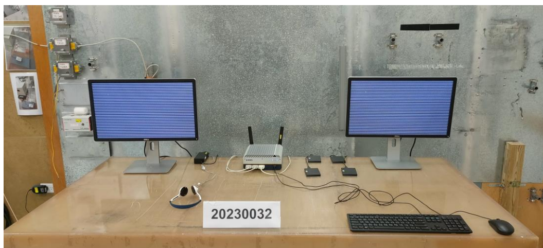
Conducted Emission Test Set up-Front View of AC mains power port
