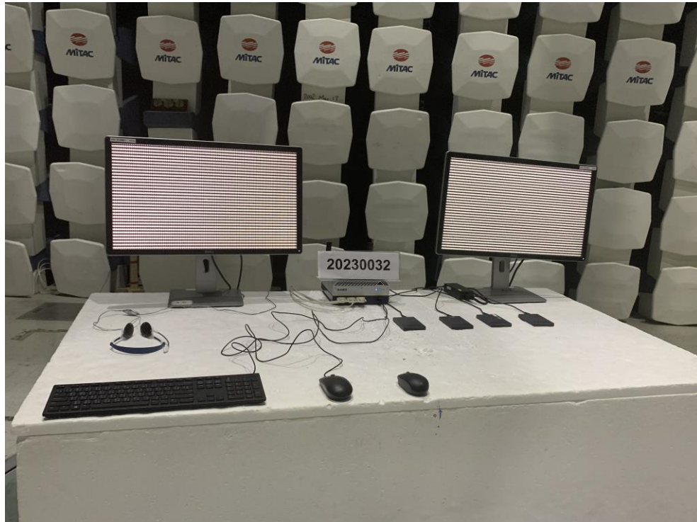
Radiated Emission Test Set up (Below 1GHz)-Front View
