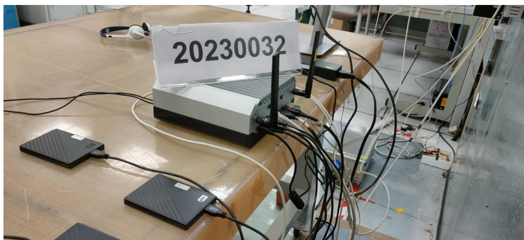
Conducted Emission Test Set up-Rear View of AC mains power port
