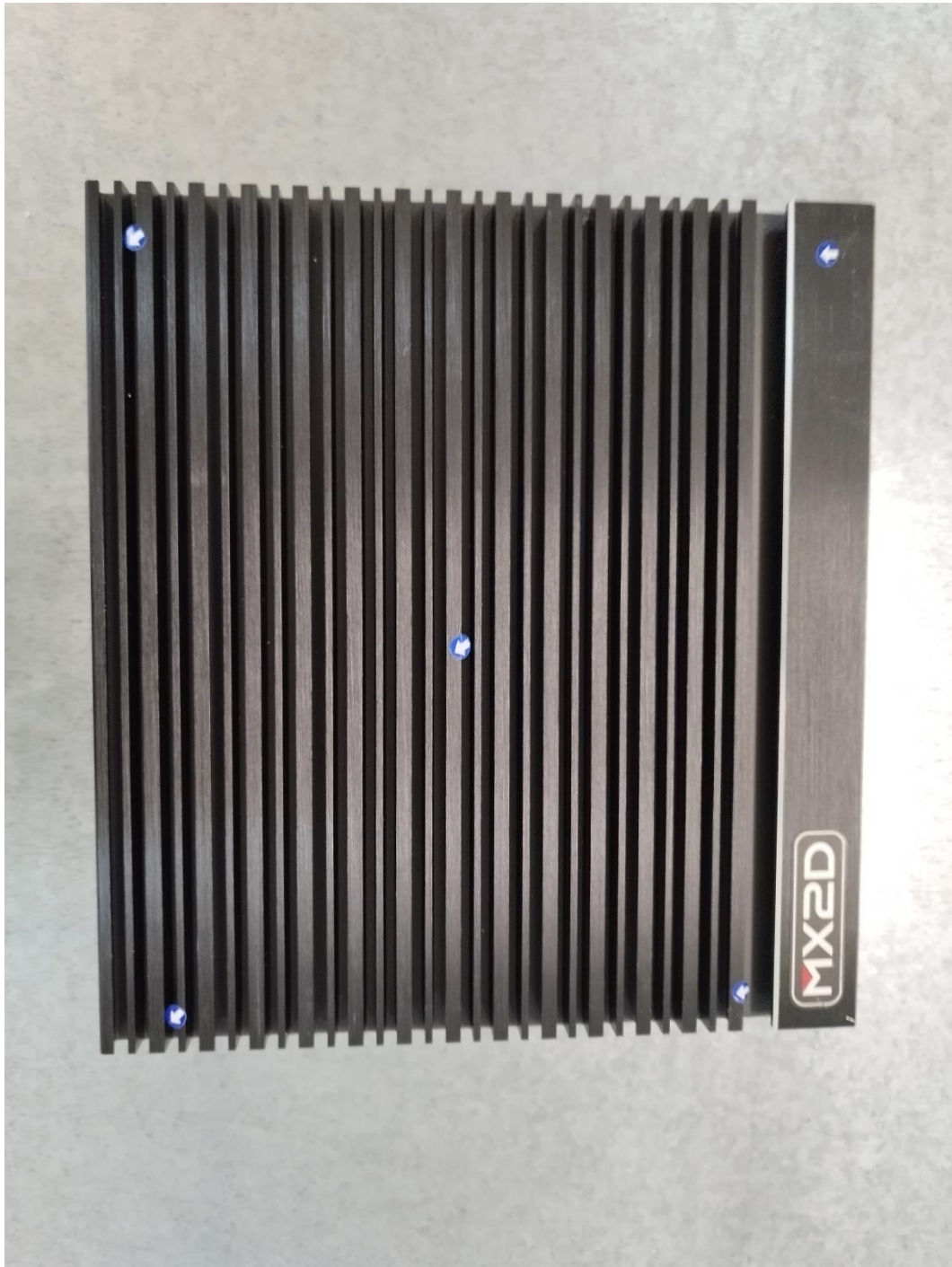
Contact Discharge Test Point-Top View
