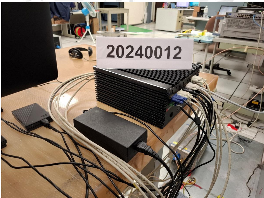
Conducted Emission Test Set up-Rear view of Power Port
