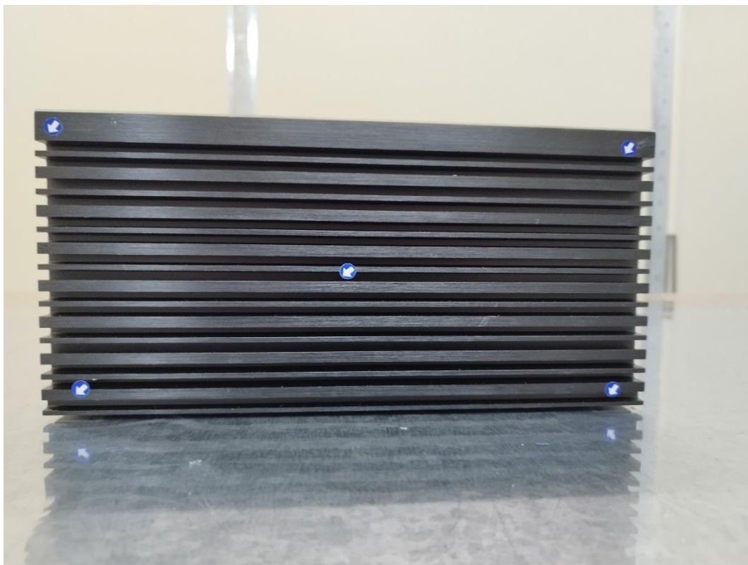
Contact Discharge Test Point-Left View
