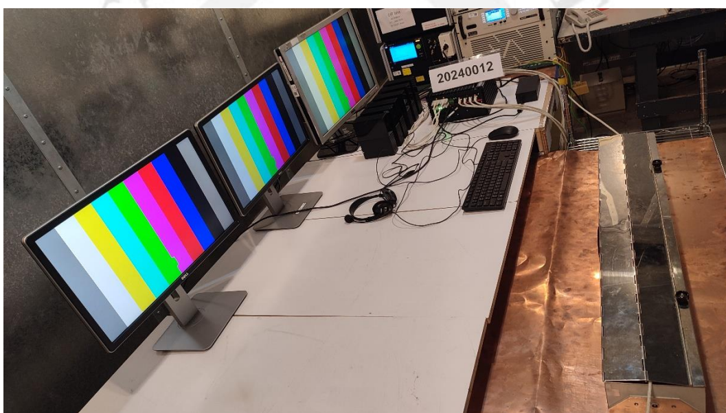
Electrical Fast Transient/Burst Set up-Signal Port
