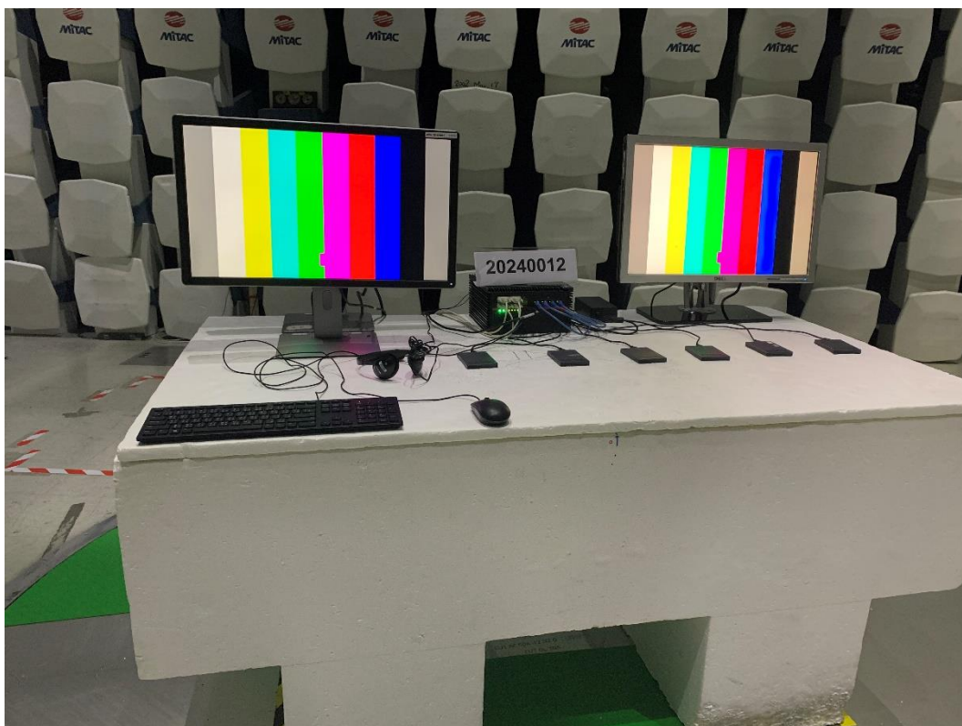
Radiated Emission Test Set up(Below 1GHz)-Front View
