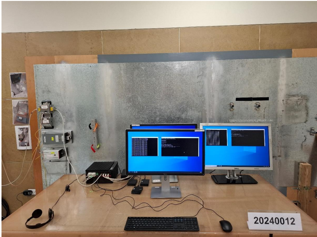
Conducted Emission Test Set up-Asymmetric mode(1Gbps)
