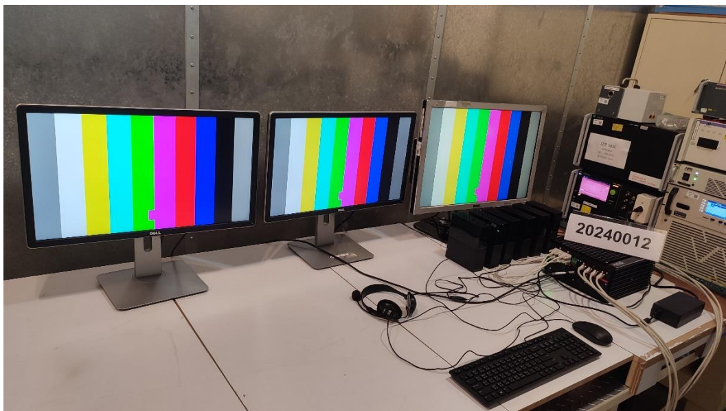
Surge Test Set up-Power Port
