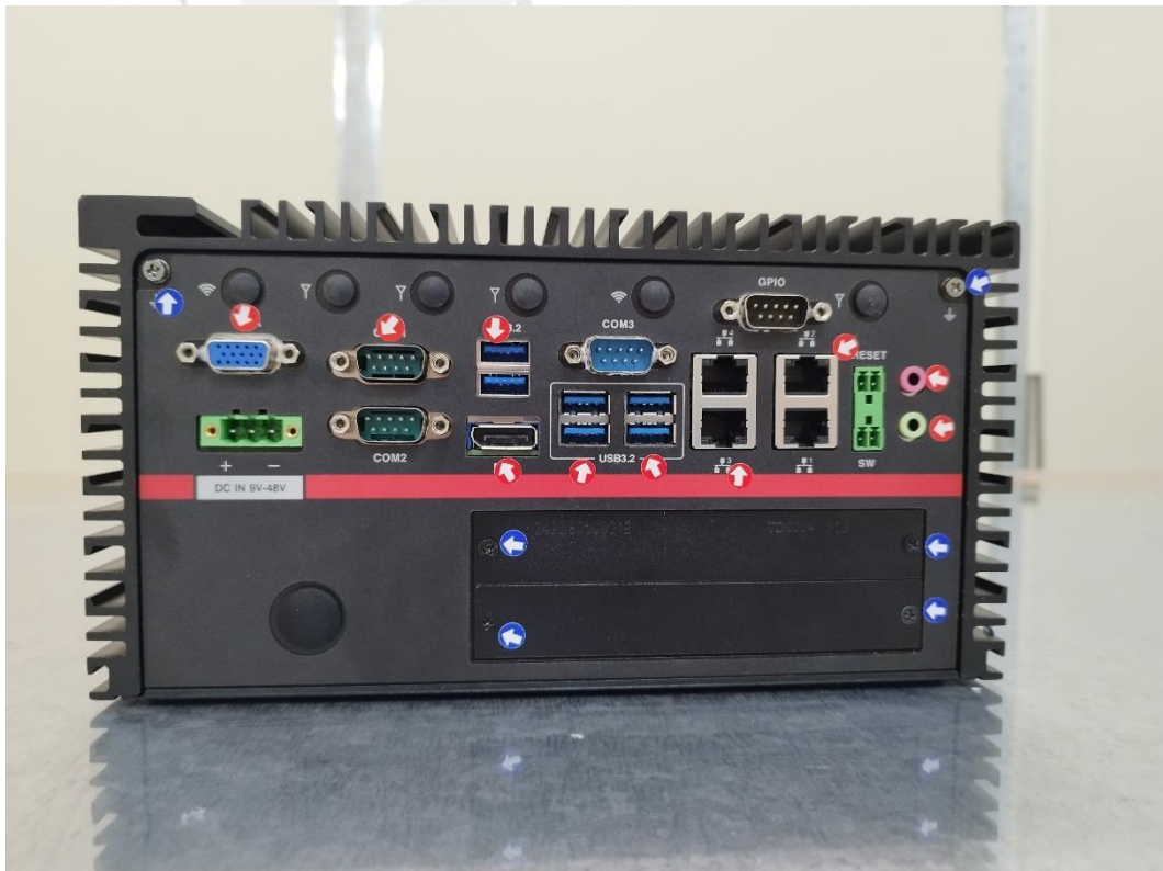
Air and Contact Discharge Test Point-Rear View
