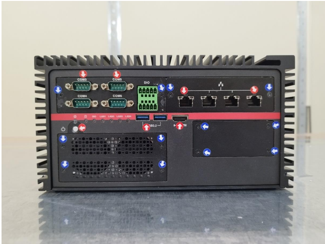
Air and Contact Discharge Test Point-Front View
