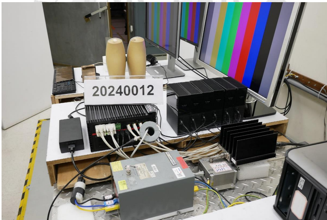
Conducted Immunity Test Set up-Rear View of Power Port
