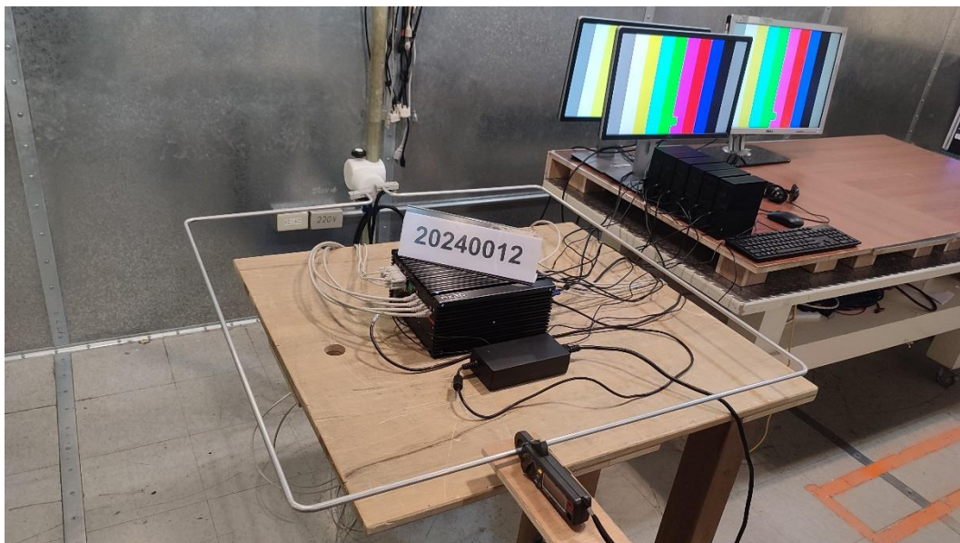
Power Frequency Magnetic Field Test-Horizontal View
