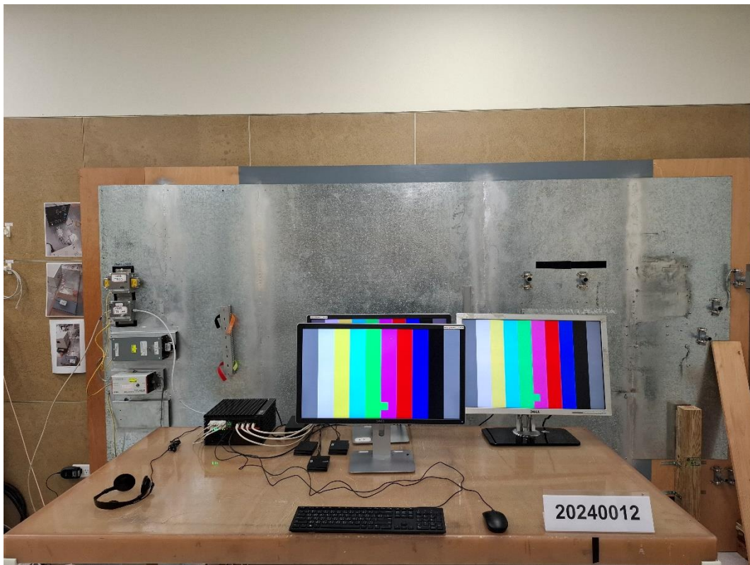
Conducted Emission Test Set up-Front view of Power Port
