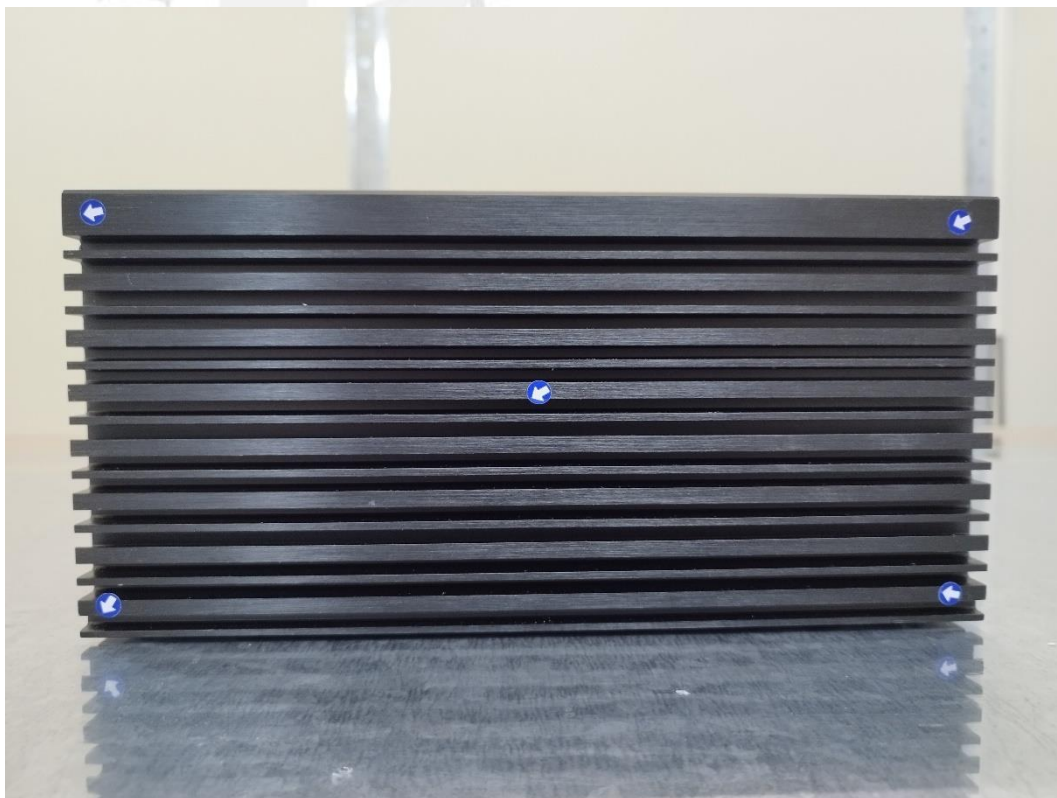
Contact Discharge Test Point-Right View
