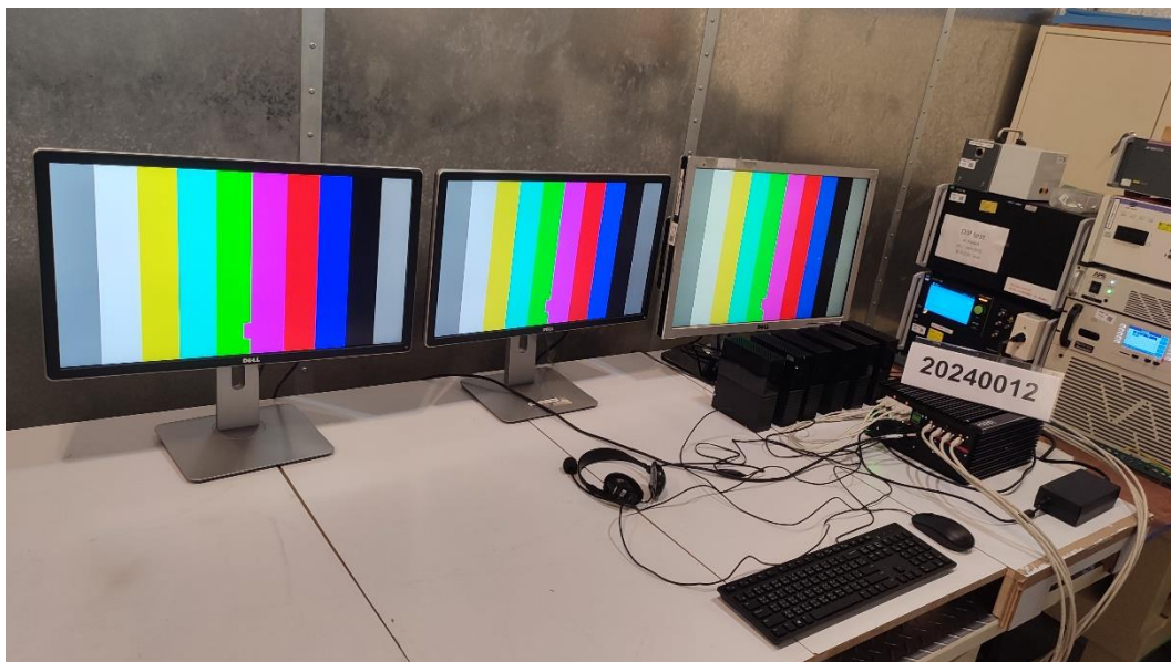
Electrical Fast Transient/Burst Set up-Power Port
