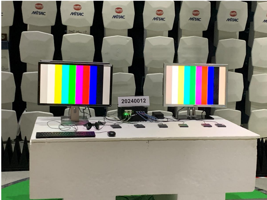
Radiated Emission Test Set up(Above 1GHz)-Front View
