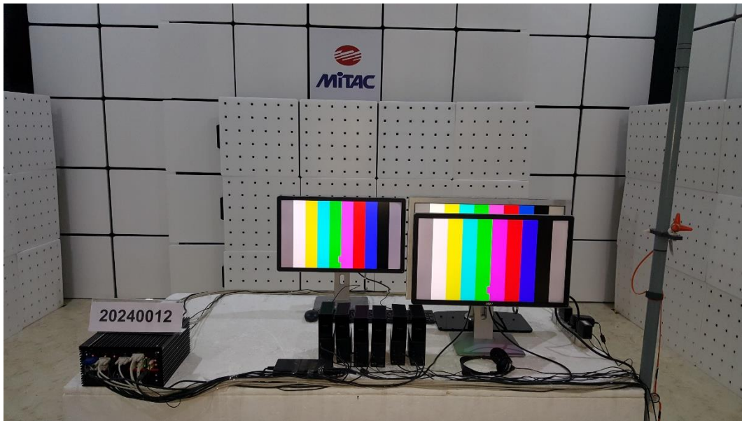
Radiated Susceptibility Test Set up-Front View
