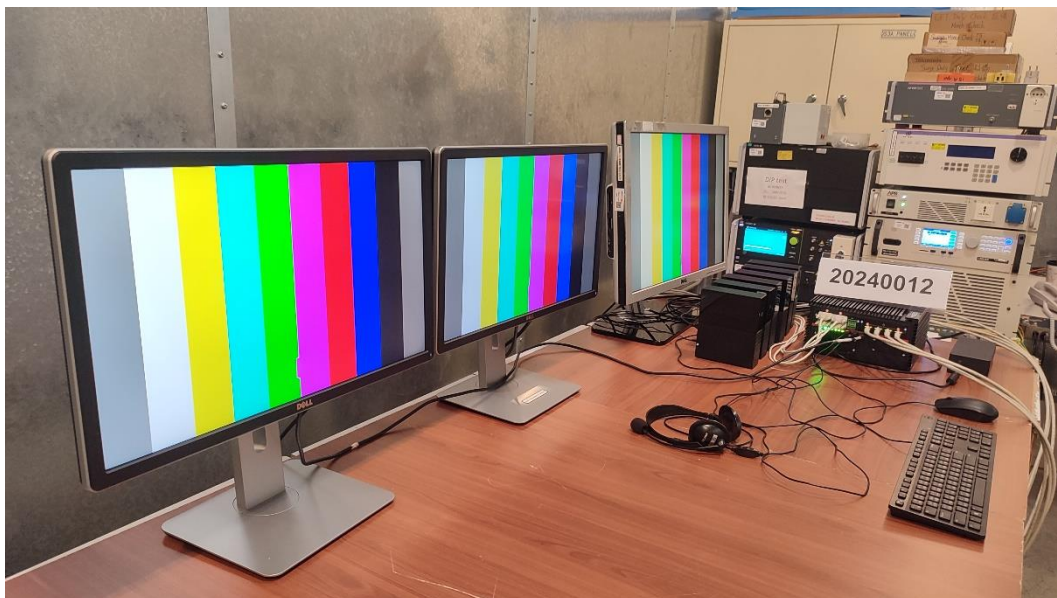
Voltage Dips Test Set up
