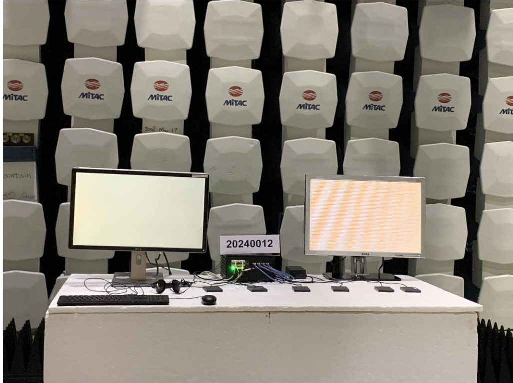
Radiated Emission Test Set up(Above 1GHz)-Front View
