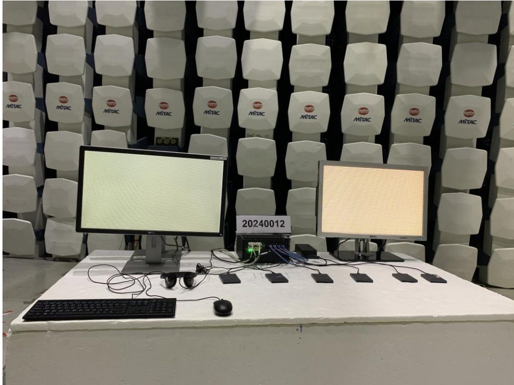
Radiated Emission Test Set up(Below 1GHz)-Front View
